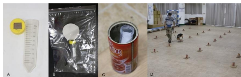
Figure 1. (A) A 50 mL centrifuge tube with a 1.7 \times 1.7 cm 2 square copper sieved cap. (B) One filter paper and the centrifuge tube with live RIFA inside were put together into a plastic zip bag ( 28 \times 42 cm 2 ) and sealed. (C) The caps of the tubes with treated or untreated papers were opened one at a time and randomly placed into metal cans for dog detection. (D) The scent lineup method was applied in a work room.
