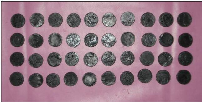
Figure 1: Forty samples of wax pattern of dimension 10 mm diameter and 2 mm thickness
