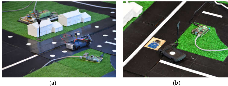
Figure 20. Lab traffic model with RFID infrastructure: (a) a vehicle equipped with RWD crossing an intersection and turning right; (b) a vehicle with RFID transponder passing over RWD.
