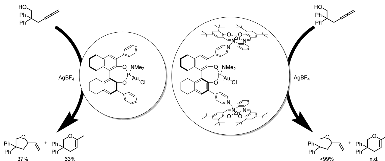
Figure 14. Gold catalyzed ring-closing reaction selectively produces the five-membered ring product when an encapsulated catalyst is applied.
