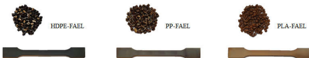
Figure 5. Picture of prepared granules of the FAEL polymer blends together with dumbbell samples for tensile testing. Lignin ester polymer blends in HDPE matrix (left), PP matrix (center), and PLA matrix (right).
