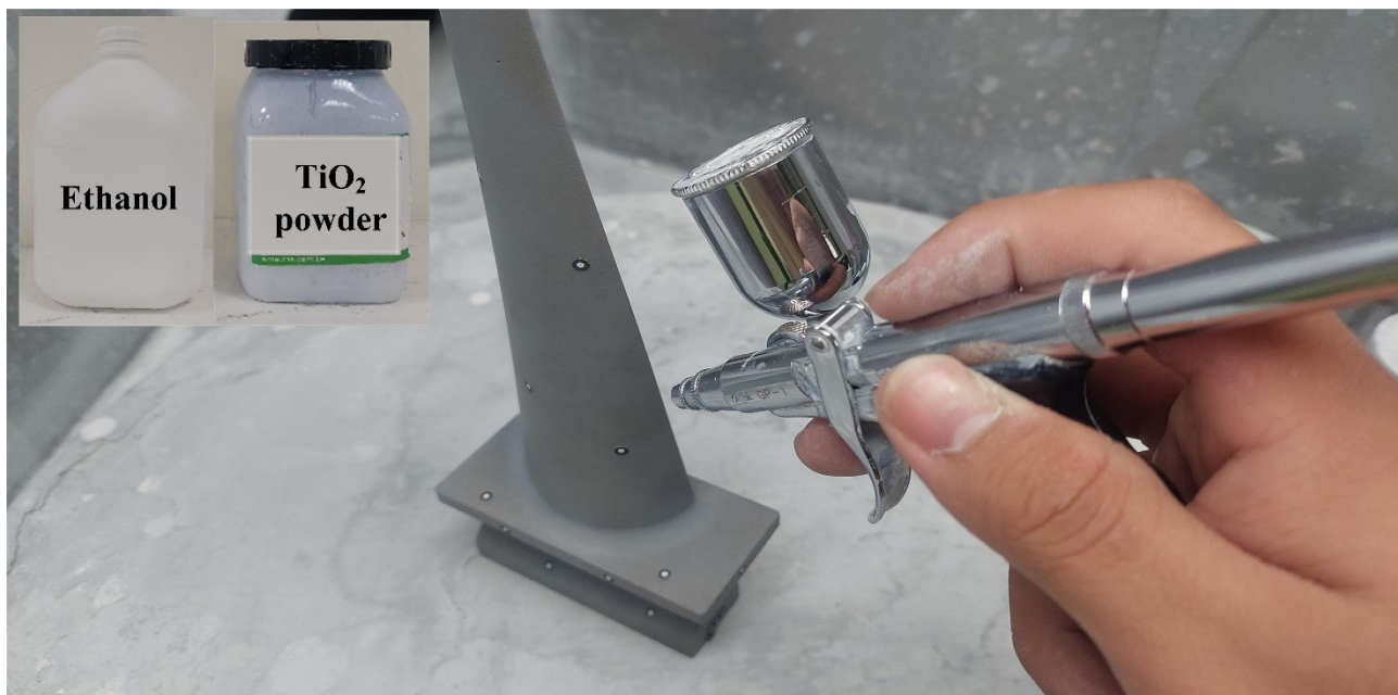
Figure 4. Situation of object sprayed with mixture of \text{TiO}_2 powder and ethanol.
