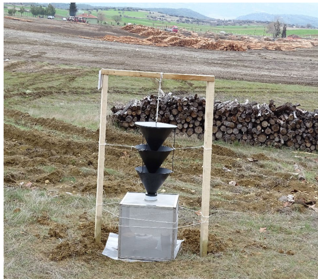
Figure 2. Insect collecting cage system integrated into Scandinavian type three funnel traps.
