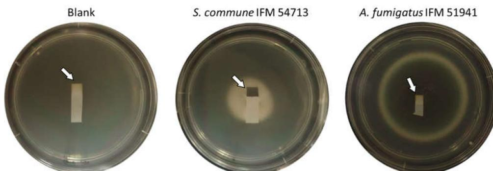
**Figure 4.** Detection of H<sub>2</sub>S using lead acetate paper. Lead acetate paper appearance exposed in a non-inoculated plate (left) and to VOCs from *S. commune* IFM 54713 (middle) and *A. fumigatus* IFM 51941 (right) for three days under 35 °C.
