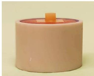
**Figure 2.** Representative image of a bonded specimen before testing.
