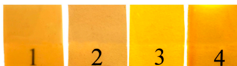
Figure 1. Optical images of membranes: (1) TPEQ-ODPA (polyimide based on 1,4-bis(4-aminophenoxy) benzene with 4,4'-oxydiphthalic anhydride); (2) Prepared mixed-matrix membrane (MMM) with TPEQ-ODPA (TPEQ-ODPA-S); (3) PMDA-ODA (poly(4,4'-oxydiphenylenepyromellitimide)); and (4) prepared MMM with PMDA-ODA (PMDA-ODA-S).
