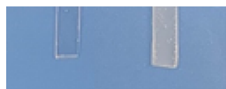
Figure 9. Optical image of DGEBA-MHHPA cured with ZIF-8 (left) and \alpha -ZrP-2MIm (right).
