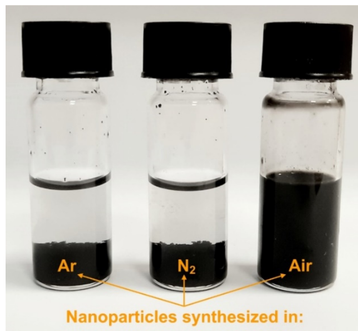
Figure 9. Photo of the prepared suspensions (nano-inks) with Pt nanoparticles (25 wt.%) dispersed in ethylene glycol (EG) with polyvinylpyrrolidone (PVP).
