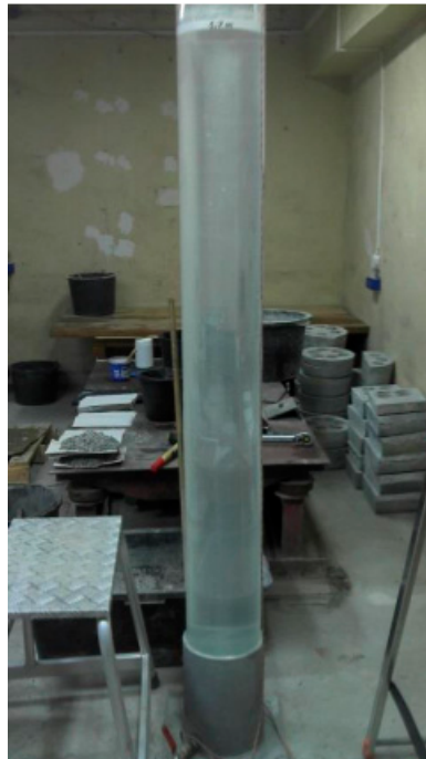
Figure 4. The pipe for wash-out loss testing.
