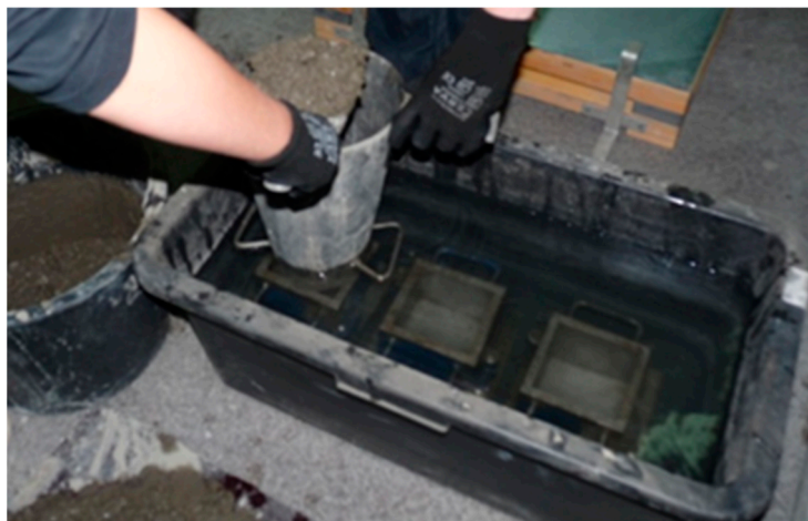
Figure 2. Preparation of specimens for strength testing.
