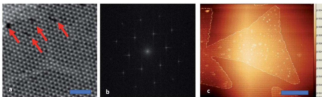
Fig. 3 The 1L MoS 2 irradiated at 1 \times 10^{14} He + ions per cm 2 dose. (a) HAADF-STEM image; scale bar is 4 nm; the red arrows indicate single and double sulfur terminations. (b) Fourier transform of STEM image. (c) AFM topography; scale bar is 4 \mu m.
