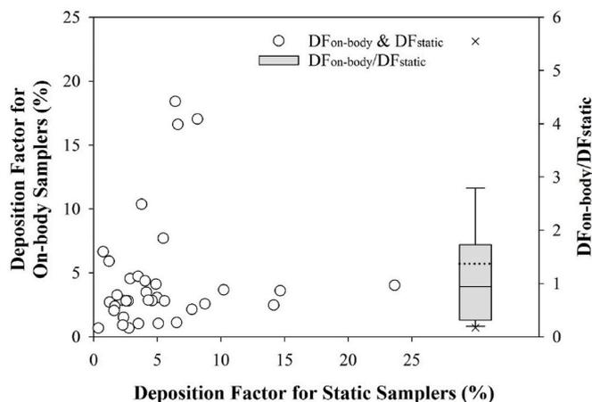
Fig. 9. Comparison of particle deposition factors between on-body samples and static samples.
