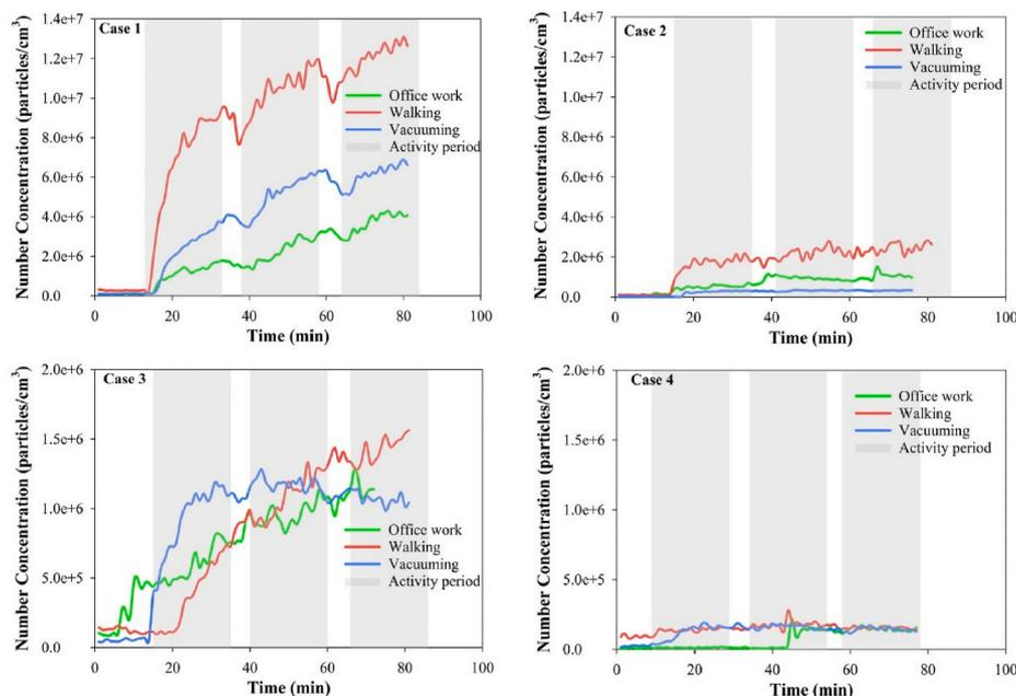
Fig. 4. The average airborne particle number concentration measured by three particle counters in the size range of 2.5–5.0 μm in the first scenario. Cases 1, 2, 3, and 4 represent: dirty floor for carpet, dirty floor for VCT, clean floor for carpet, and clean floor for VCT, respectively. It should be noted that the graphs for cases 1 and 2 have a different scale than the graphs for cases 3 and 4. The gray area represents the activity periods.
