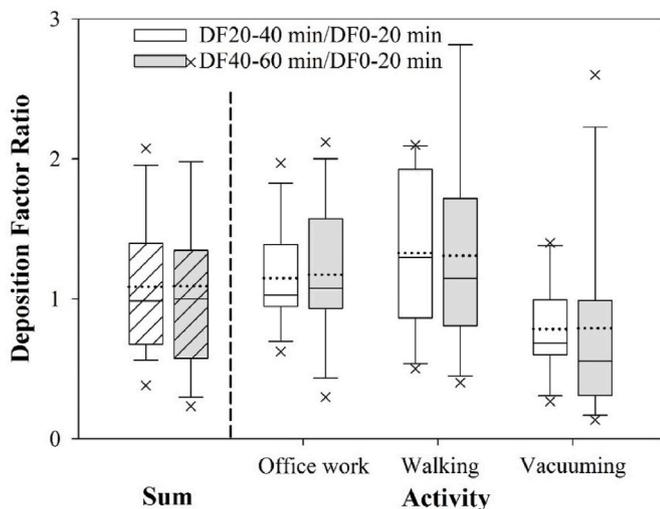
Fig. 6. The effect of the sampling period on the particle deposition factor.
