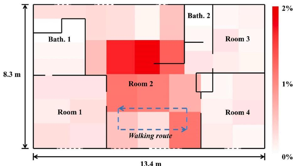
Fig. 8. The distribution of resuspended FPs from clothing in the test house. The percentage is the particle resuspension factor.
