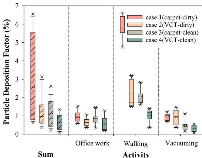
Fig. 5. The effect of flooring types and conditions on the particle deposition factor. The × symbols below and above the boxes are outliers (1<sup>st</sup> and 99<sup>th</sup> percentiles); the lines below and above the boxes are the 5<sup>th</sup> and 95<sup>th</sup> percentiles; the bottom and top of the boxes are the 25<sup>th</sup> and 75<sup>th</sup> percentiles; and the solid lines in the boxes are the medians and the dotted lines are the averages.
