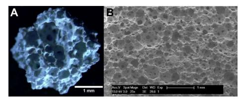
**Figure 1.** (**A**) A stereomicroscopy image of a PermaBone<sup>®</sup> hydroxyapatite granule. (**B**) A scanning electron microscopy image of pre-granulated PermaBone<sup>®</sup> hydroxyapatite.
