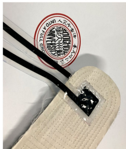
Figure A6. Photo of placing of the sensor on the insole.
