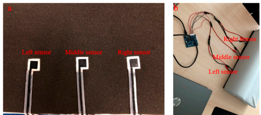
Figure A7. (a) Three flexible sensors on the pillow, (b) the test circuit diagram of our smart pillow.
