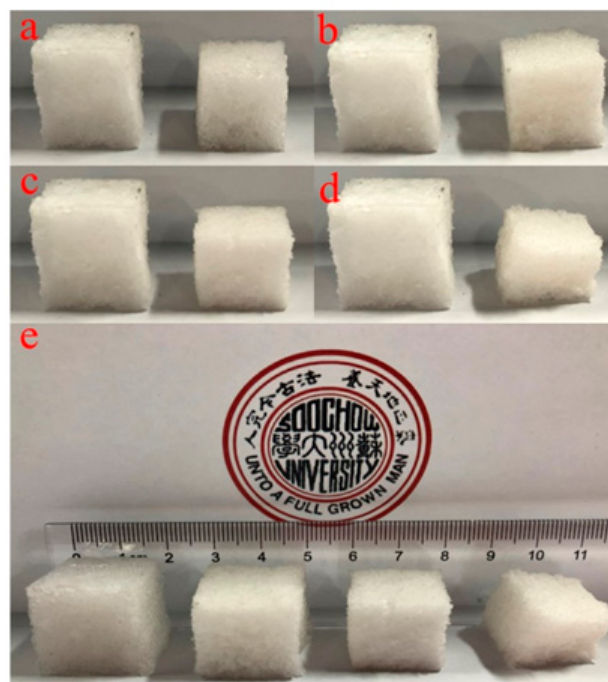
Figure A1. The images of the PDMS sponge with different mass fraction of CAM. (a) m_{\text{PDMS}}:m_{\text{CAM}} = 1:3 , (b) m_{\text{PDMS}}:m_{\text{CAM}} = 1:5 , (c) m_{\text{PDMS}}:m_{\text{CAM}} = 1:7 , (d) m_{\text{PDMS}}:m_{\text{CAM}} = 1:9 , (e) the images of four PDMS sponges.
