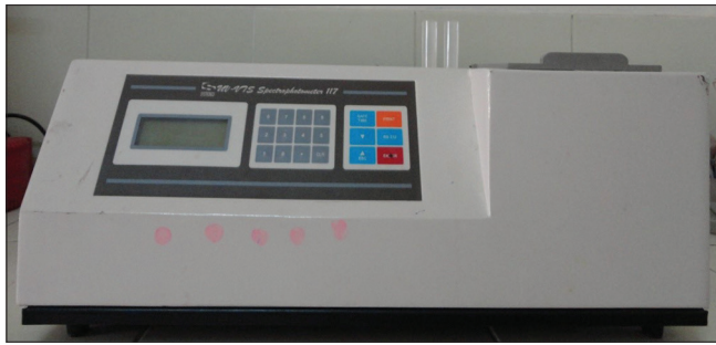
Figure 2: Spectrophotometer used for salivary thiocyanate estimation (UV-VIS Systronics 117)
