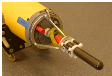
Figure 14. NeXOS A1 Hydrophone integrated on the SeaExplorer glider as payload.
