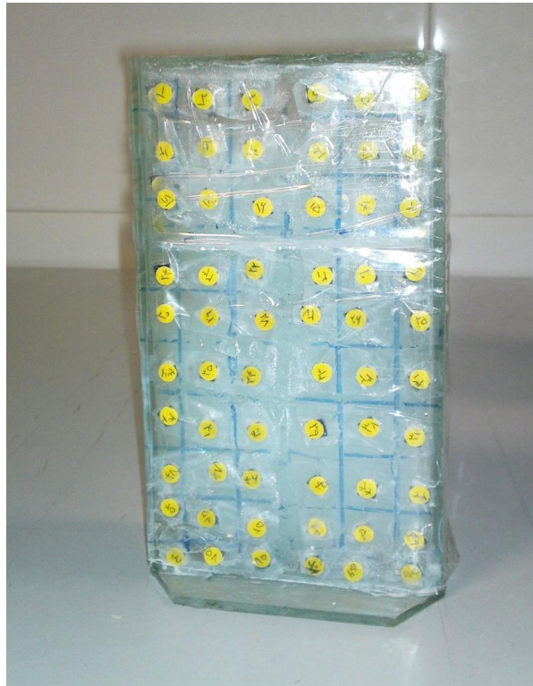
FIG. 1. The phantom used for gel dosimetry with the TLD chips on the surface.
