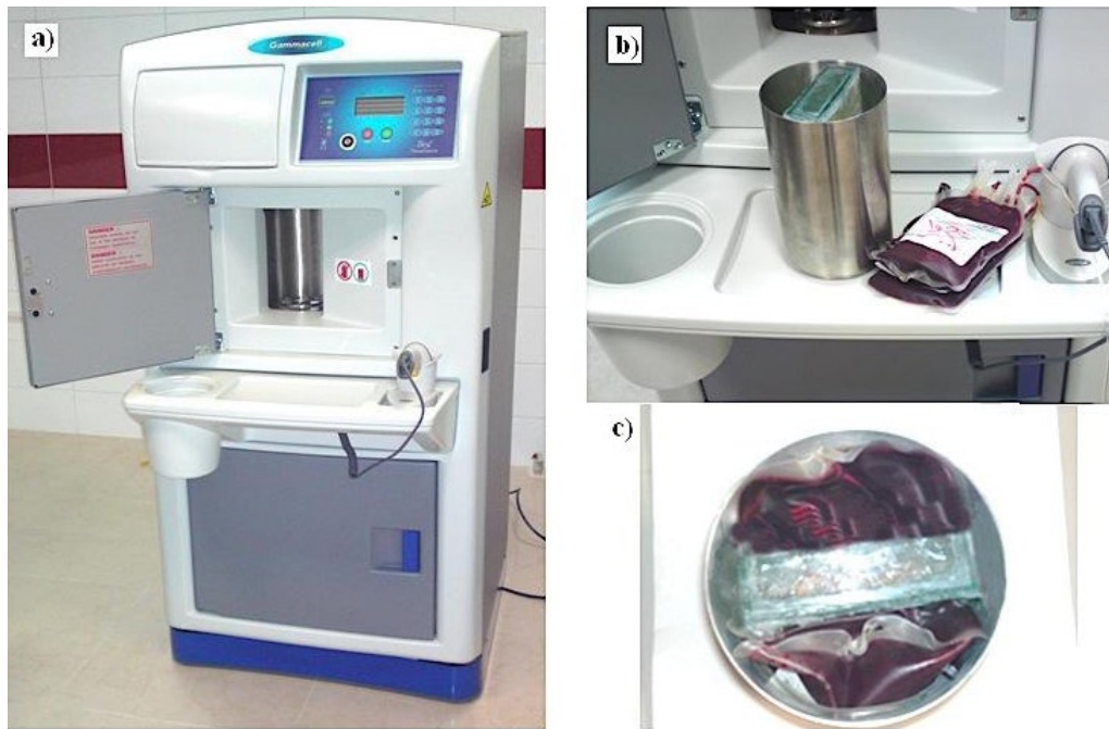
FIG. 2. The blood irradiator (a), gel phantom (b), and gel phantom inside the blood container ready to be irradiated (c).
