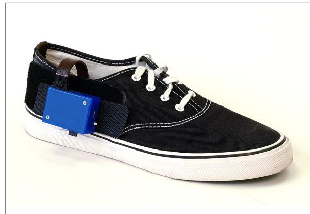
Figure 1. Footpressure ITE System: a device fixed to the outer surface of a shoe that registers and transmits data.
