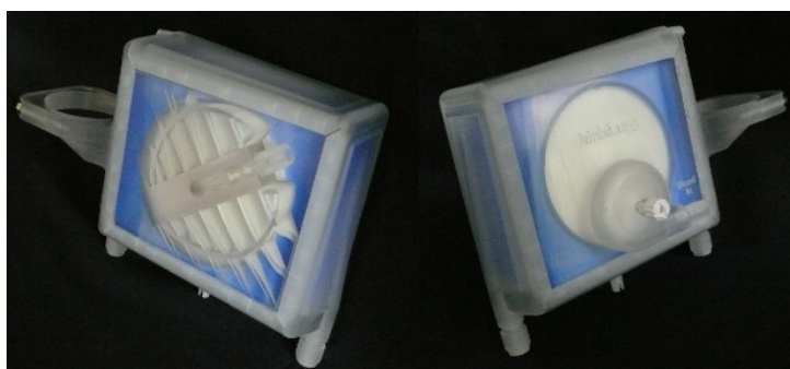
Figure 3. Novel portable, stacked, and centrifugal potted membrane oxygenator front and back.
