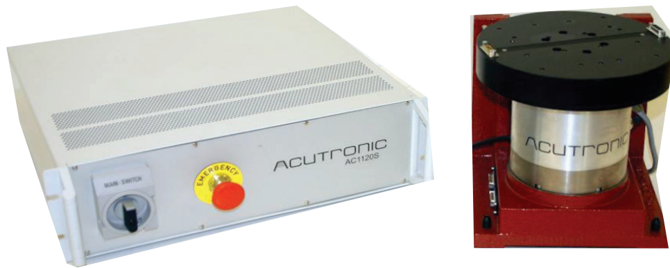
Figure 3. Instrumented turntable used in the complex calibration. The Acutronic AC11205 has a precision of 0.0001% over 360 degrees. A custom aluminum block is mounted on top of the turntable with screws to ensure proper sensor placement and orientation.
