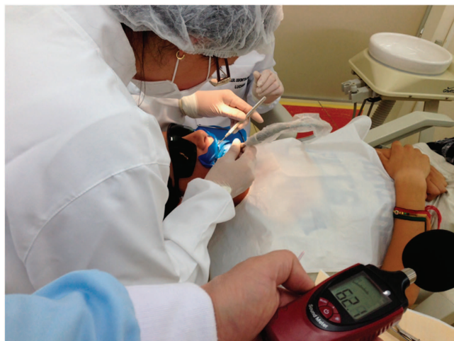
Figure 1. Measurement of noise using the decibelimetre.
