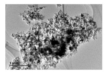
**Figure 1.** Transmission electron mocroscopy (TEM) image of nano-Al<sub>2</sub>O<sub>3</sub> in the exposure solution. Nano-Al<sub>2</sub>O<sub>3</sub> was agglomerated to large particles (about 1000–3000 nm).
