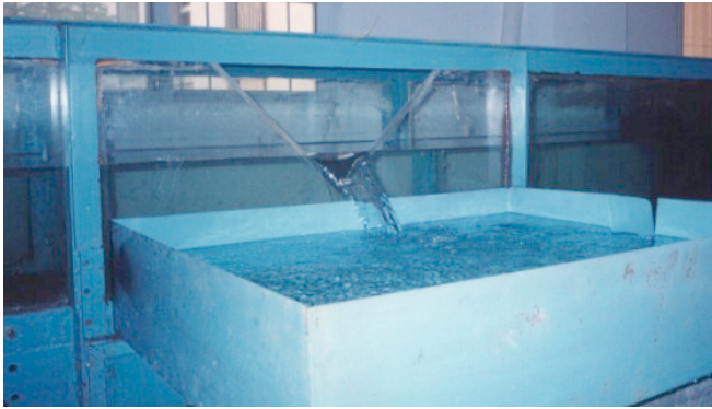
Fig. (1). Experiment scene of side-weir flow.
