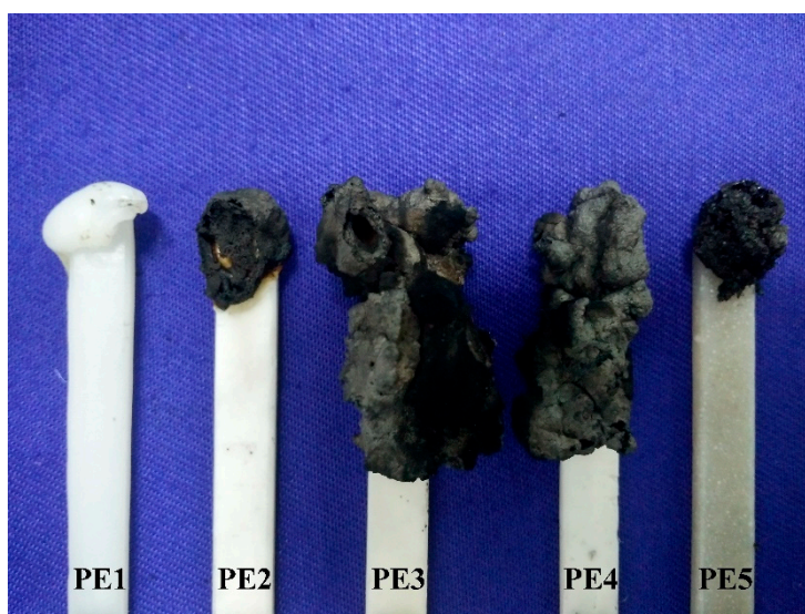
Figure 3. Photos of char residues after LOI test for HDPE and HDPE/IFR composites.
