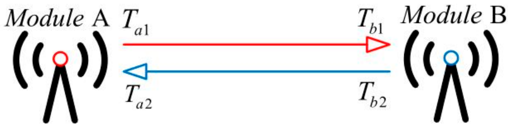
Figure 1. Two way-time of flight ranging principle.
