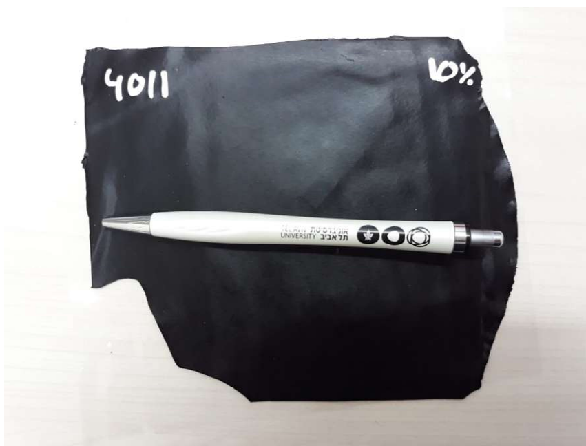
Figure 1. Vulcanized plate of VMQ with 10 wt.% of MWCNT. Pen to scale.
