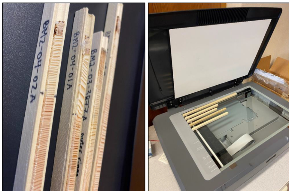
Fig. 3. (A) Prepared, cleaned cores ready for scanning. (B) Cores placed on the scanner just before scanning.
