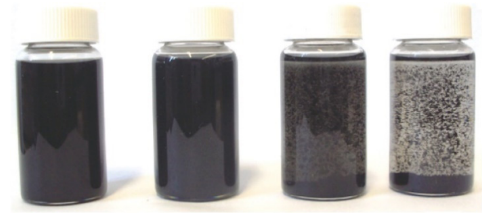
Figure 9. Photographs of various CNT dispersion in dilute epoxy solution (xylene-butanol (1:1) mixture) when the mixture was allowed to settle for 6 h. From left to right: CNT-ODA; CNT-OH; CNT-COOH and CNT-raw Copyright 2010, American Chemical Society. Reprinted with permission from Ref. [193]. Copyright 2004 American Chemical Society.
