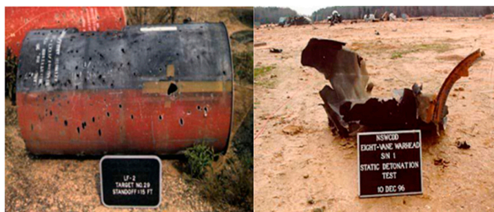
(a) Comparison of target damage between inert damage element (left) and active damage element (right)
