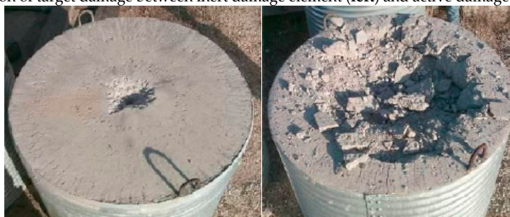
(b) Damage comparison of inert liner (left) and active liner (right) to target hole
