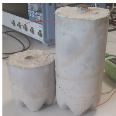
Figure 12. Reinforced concrete structures with 10 and 20 cm long steel with a concrete cover thickness of 40 mm.
