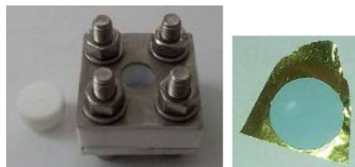
Fig. 5 Vessel used for preparation of targets by gravimetric sedimentation ( left ) and a 3 \text{mg}/\text{cm}^2 \text{Nb}_3\text{O}_2 layer on an Au backing, deposited by this method from a suspension in diluted epoxy resin
