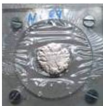
Fig. 2 An S target pellet ( left ) prepared by powder pressing with use of a hydraulic press ( right )
