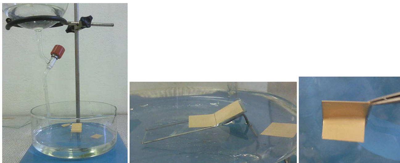
Fig. 14 Floating process used for releasing foils from the substrate and fishing on a frame
