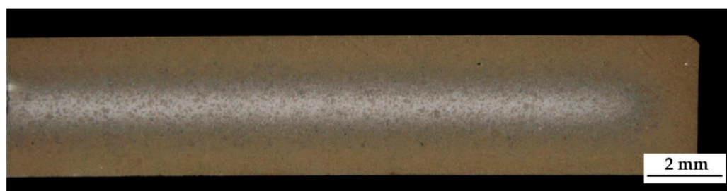
Figure 3. Macroscopic overview of the polished section of the carburized sample without hollow spheres. Color differences provide a visual idea of the hardening depth.
