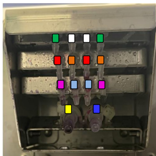
Figure 2. Arrangement of 14 nozzle tips. White: methanol, Purple: crystal violet, Brown: iodine, Light blue: acetone/ethanol, Red: Fuchsin, Green: unused, Blue: rising water, Yellow: blower.
