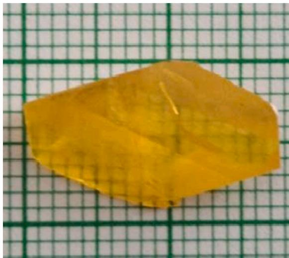
Fig. 2. Photograph of as-grown single Crystal of CHAP.
