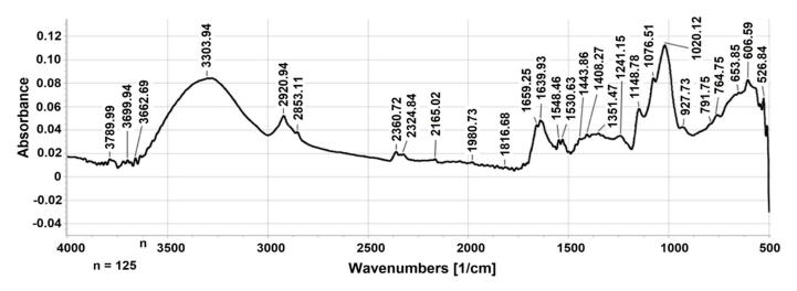
Figure 1. ATR-FTIR spectrum of MP-PSC.
