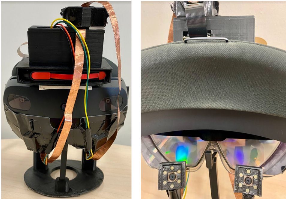
Figure 2. Front view and inside view of the camera mount attached to HoloLens 2 display.
