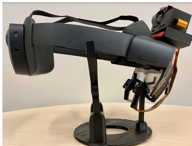
Figure 1. Side view of camera mount attached to HoloLens 2 display.
