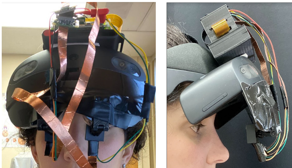
Figure 3. Front view and side view of user wearing headset camera system.
