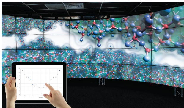
Figure 9: Platform illustration in a hybrid environment made of a 3D immersive CAVE2 system (EVL/UIC, Chicago) together with a graphical tablet for 2D analytical representation.
