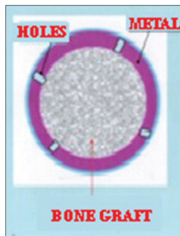
Figure 2: Bone impregnated hip screw cross section showing bone graft and staggered holes
