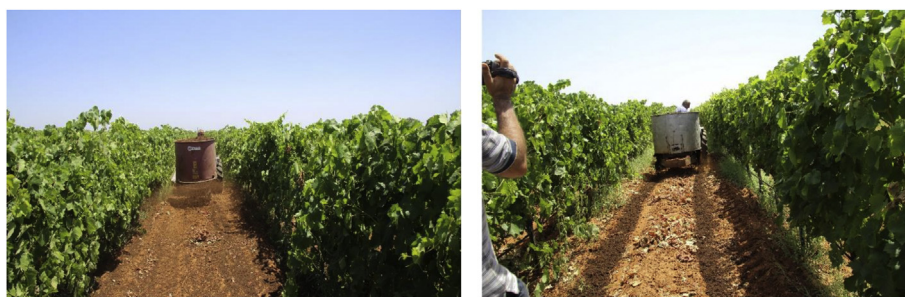
Figure 3. Spreaders used in the vineyard: broadcast spreading on the left and localised on the right.
