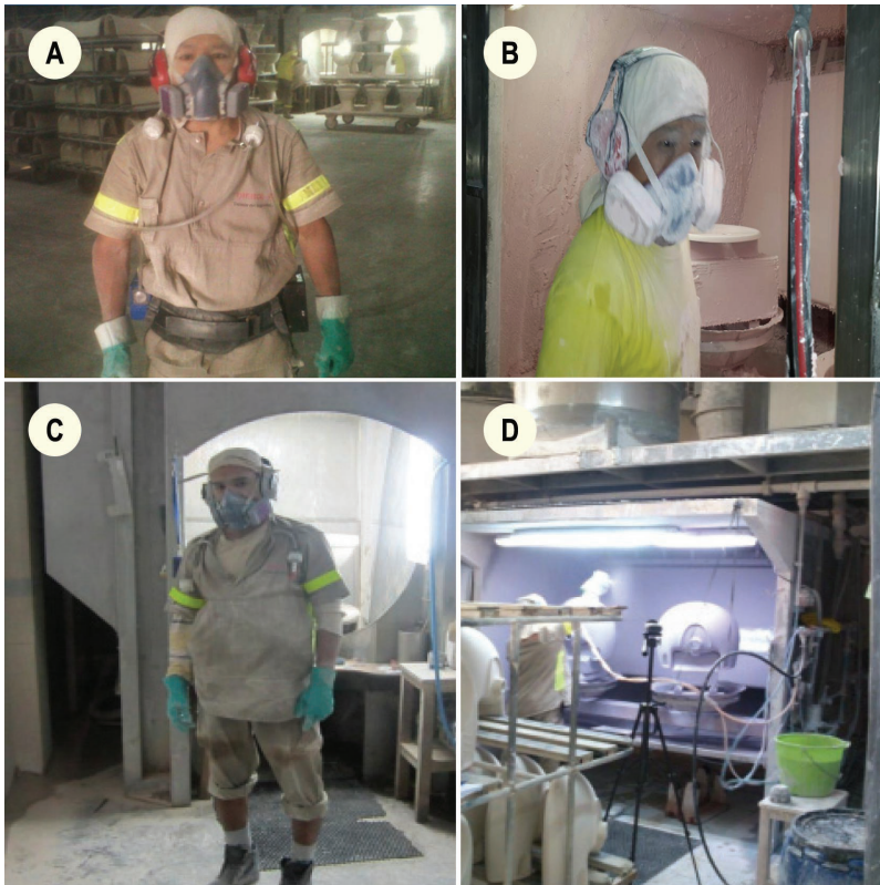
Figure 1: A typical personnel during the execution and at the end of his work activities. A) A polisher with particulate matter sampling pump whose eyebrows become white by the dust generated by the polishing of the toilets. B) An enameller whose eyebrows and the ocular perimeter become white by the particulate matter. C) A polisher with particulate matter sampling pump. The polishing booth is seen behind the employee. D) An enameller doing the lavatories enamelling process. The enamelling cabin and the mist generated are observed.
