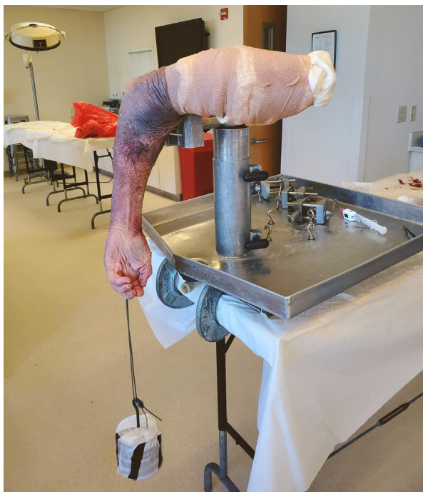
Figure 2. Photograph of the experimental design for weight suspension. The cadaveric specimen is mounted on a vice with the hand pointed downwards. The weight was suspended from the middle finger by a string with the wrist in a neutral position.
