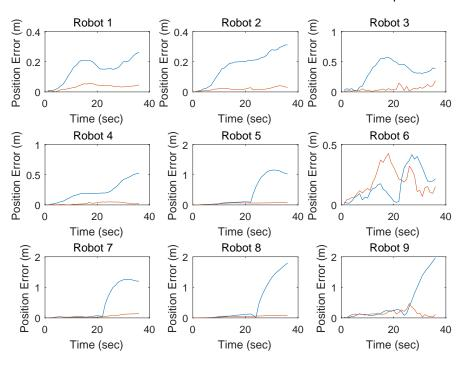
Position Error of 9 robots under Additive White Gaussian Noise and Impulse Noise
