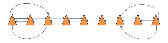
Figure 8. Communication graph for 9 robots.
