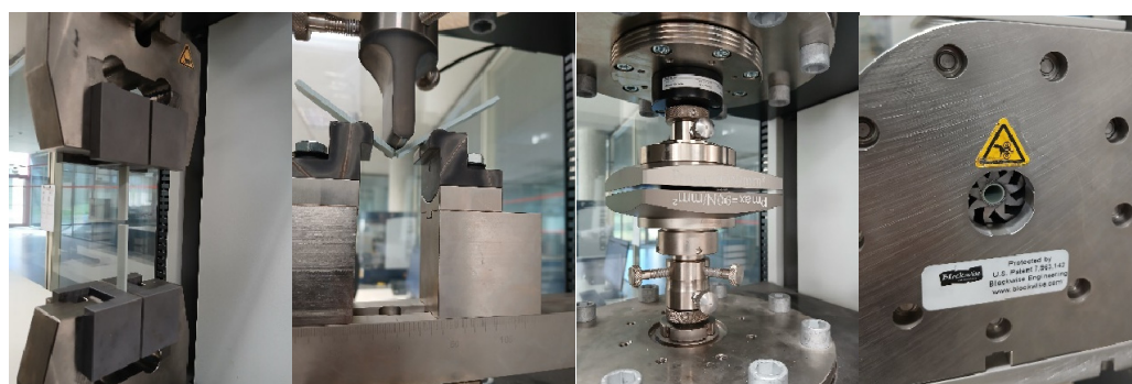
Figure 7. Tensile, flexure, axial compression and radial compression test, from left to right.
