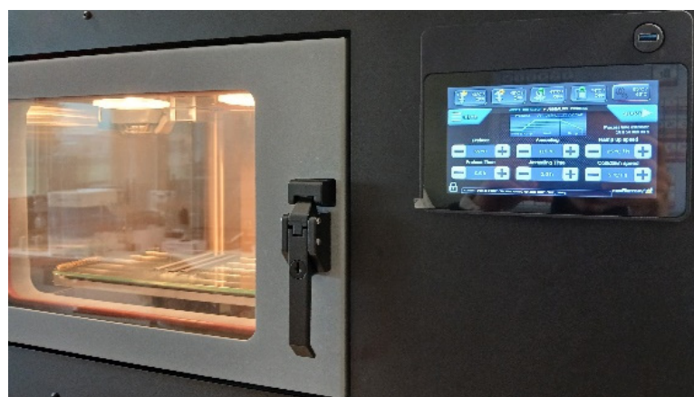
Figure 5. Annealing of PLA–Mg specimens in the Minifactory Ultra 2 printer.
