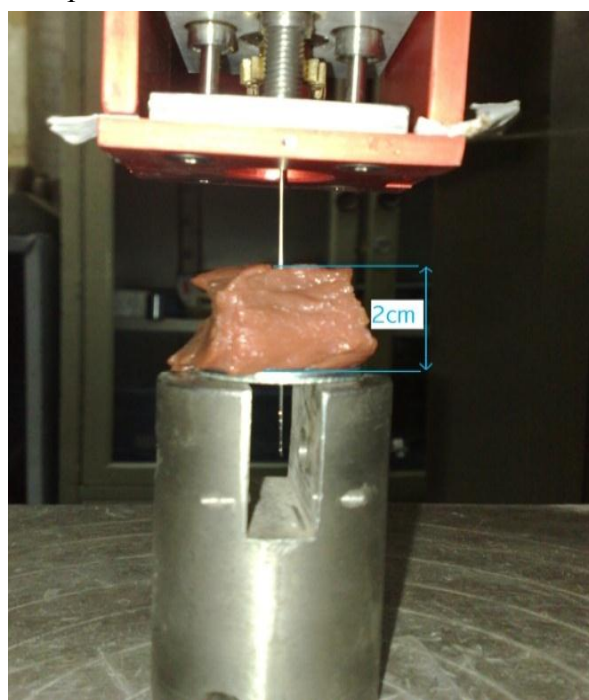
Figure 5: Deep needle insertion to definite tissue thickness in order to measure the amount of friction force
