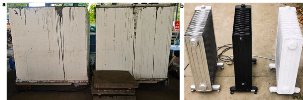
Fig. 6. Photographs of concrete model buildings (a) and electric oil heaters (b) painted with the HE, aluminium and black coatings.
