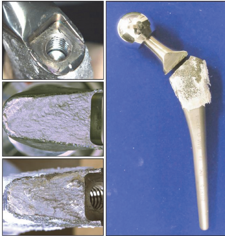
FIGURE 2: Appearance of the broken stem. Macroscopic appearance of the broken AHFIX Q stem at the base of the neck. The proximal coating area shows good bone ingrowth. The base of the neck has a sharp slot for handle attachment and the corner is not rounded but is angular.
