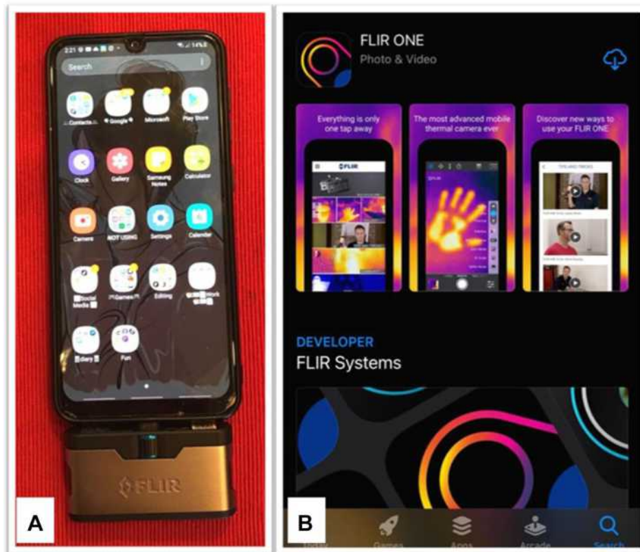
Figure 1 Showing the Flir One thermal camera connected to the smartphone (A) and operated using an application available on the Google Play store (B).
